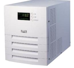
The AR-XXK automatic voltage regulator features CPU control, LCD display, IGBT inverter design, has a wide input voltage window and excellent voltage regulation with a margin of 1%. It is compatible with linear and non-linear loads, and includes overload, high voltage and low voltage protection. It also has a built-in surge suppressor (MOV), EMI & LC filters which provide pure and clean output.
