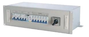
Main features include: DC input breaker, AC input breaker, AC input SPD (Class C 20kA), 6 x switched outputs with IEC60320-C14 sockets (10A max, each), 1 x bulk AC output (32A) and maintenance bypass switch (40A, make before break, 4ms transfer time).
