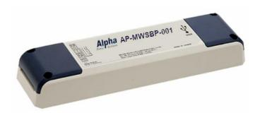
AP-MWSBP-001 is a Smart Charging Programmer, particularly for the various AP-MWNPB programmable battery charger models to configure the parameters of charging curves, such as constant current, constant voltage, float voltage and tapper current. User can easily programme the settings to accommodate the diversified batteries for simplicity and convenience with the means of a computer and the well-designed software.
